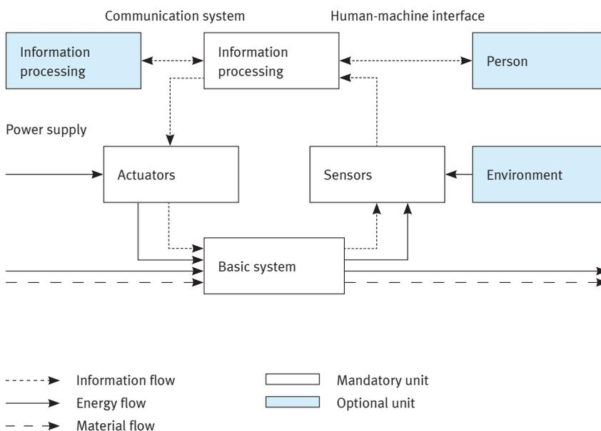
Figure 1: Basic structure of a mechatronic system<sup>1</sup>
