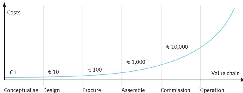
Figure 2: Rule of ten for subsequent system adaptations
