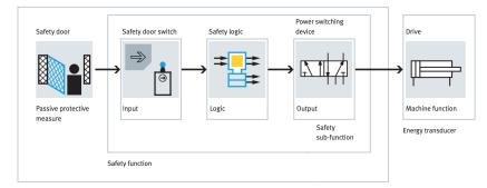
Some common examples of safety sub-functions in pneumatic and electric drive technology include:
