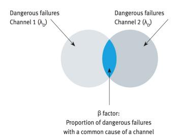
**Fault Behavior.** For category 2 safety circuits, you can assess fault behavior with a failure mode and effects analysis (FMEA) or fault tree analysis (FTA). Depending on your application and selected components, however, you may need to take additional measures to meet ISO 13849 requirements.
