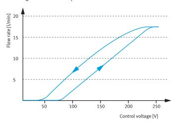
Proportionality of piezo valves: ideal actuators for higher-level control systems
